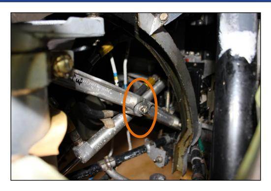
**Photo No. 1**: Linkages as found with no geometric lock in evidence.
