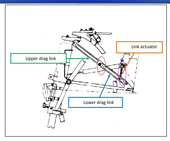
**Figure No. 1**: NLG actuation schematic showing the geometric lock (red) and down lock link (purple)
