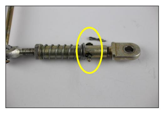
Photo No. 4: Down lock link elongated pin holes and improper spring loading.
