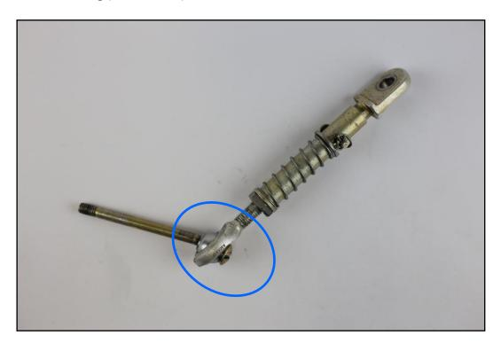
**Photo No. 3**: Failure in bending of the down lock link bolt.
