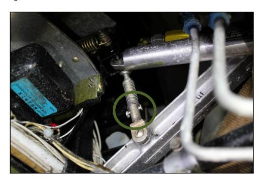
Photo No. 2: Down lock link crush damage at the pinholes.
